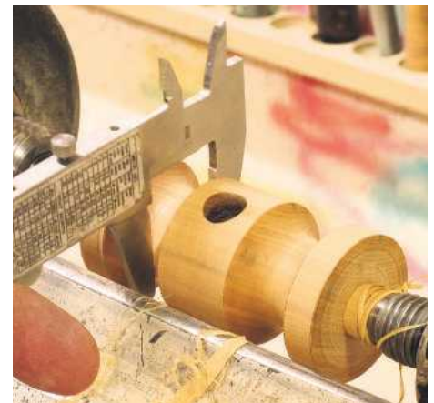
▲ Pic.24 Use the Verniers to check that both grooves are the same depth. Go down to about half the diameter, making these as accurate as possible
